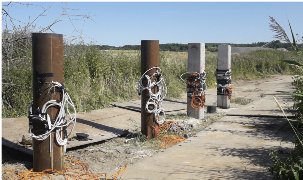
Fig. 4. Photo of test piles after completed installation.
